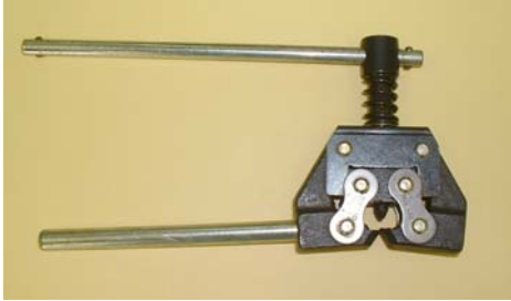
Figure 402 Hand disassembly tool - commercially available
