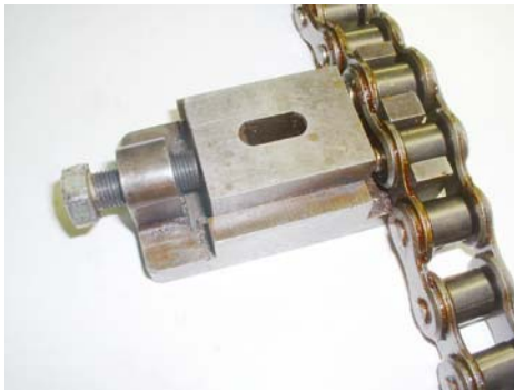
Figure 403 Homemade disassembly block for special applications.
