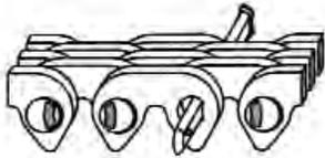
2. Insert a drilled connecting pin.
